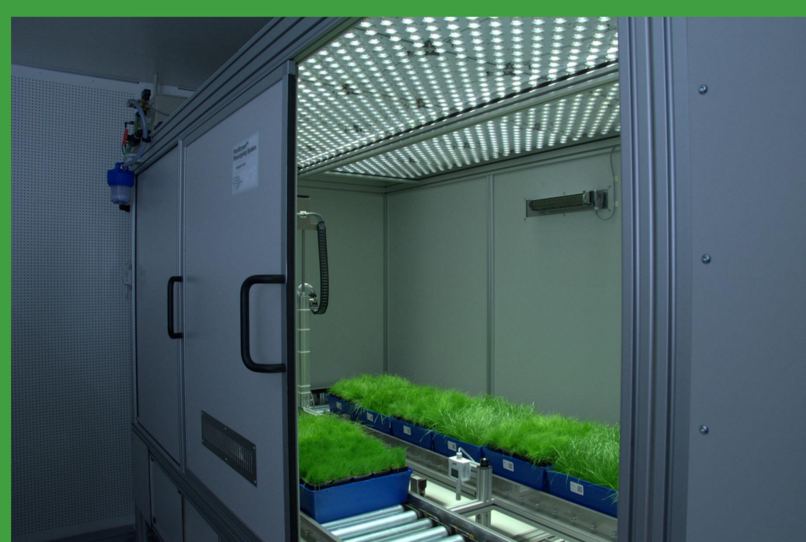
PlantScreen™ Compact System for automated phenotyping of up to 320 small- and mid-size scale plants in controlled environment.
